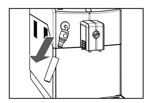
Warning! Remove the "Intenza" filter before adding the descaling solution.
