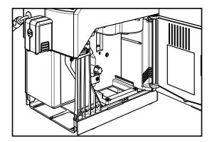
8 Insert the coffee residues drawer in its seat and ensure that it is correctly in place.
