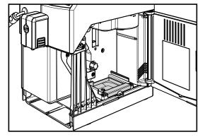
If the coffee residues drawer is not correctly positioned, the brew group may not fit into the machine.
