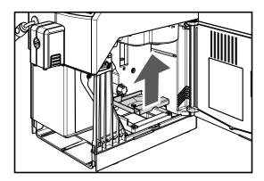
7 Clean the inside of the machine with a damp cloth.
