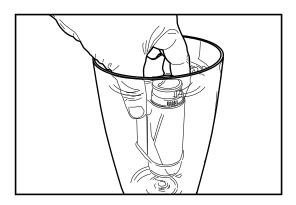
3 Remove the tank from the machine and empty it. Remove the small white filter from the tank and store it in a dry place sheltered from dust.
