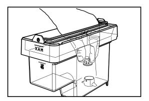
4 Put the filter into the empty tank. Press it to its limit stop.
