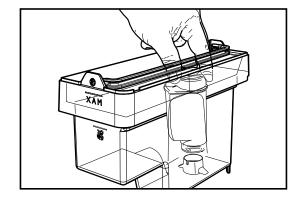
5 Fill the tank with fresh drinking water and reinsert it into the machine.
