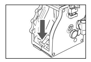
11 Make sure that the hook which locks the Brew Group is in the correct position; to check its position firmly press the "PUSH" button.
