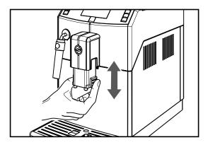
Manually move the dispensing spout up or down to adjust its height.
