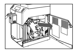
4 Remove the Brew Group: pull it by the handle and press the «PUSH» button. The Brew Group must be washed with lukewarm water only. Do not use detergent.
